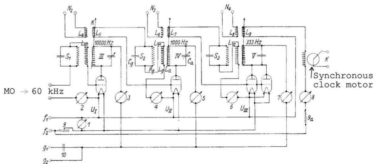
**Fig.3:** The divider circuit of the PTR clocks (1934)
