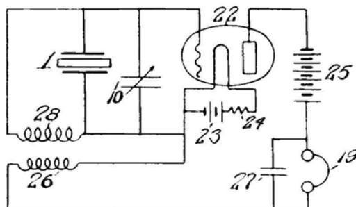
**Fig. 1:** Cady's first quartz oscillator application
