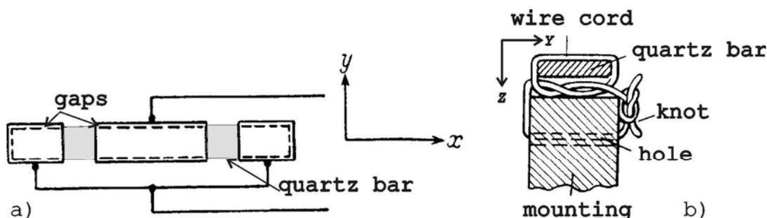
**Fig.4:** a) The quartz bar and its electrodes
