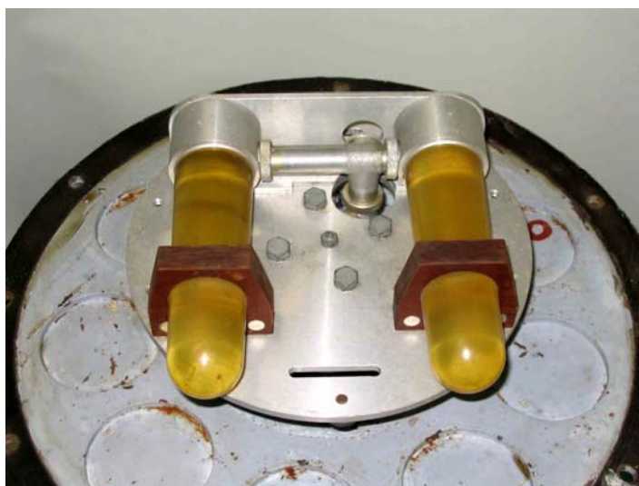
Figure 2: The shape of the Naxos antenna-arrangement is clearly visible. (Navy type ZM 290M, with its Perspex radome being removed)
