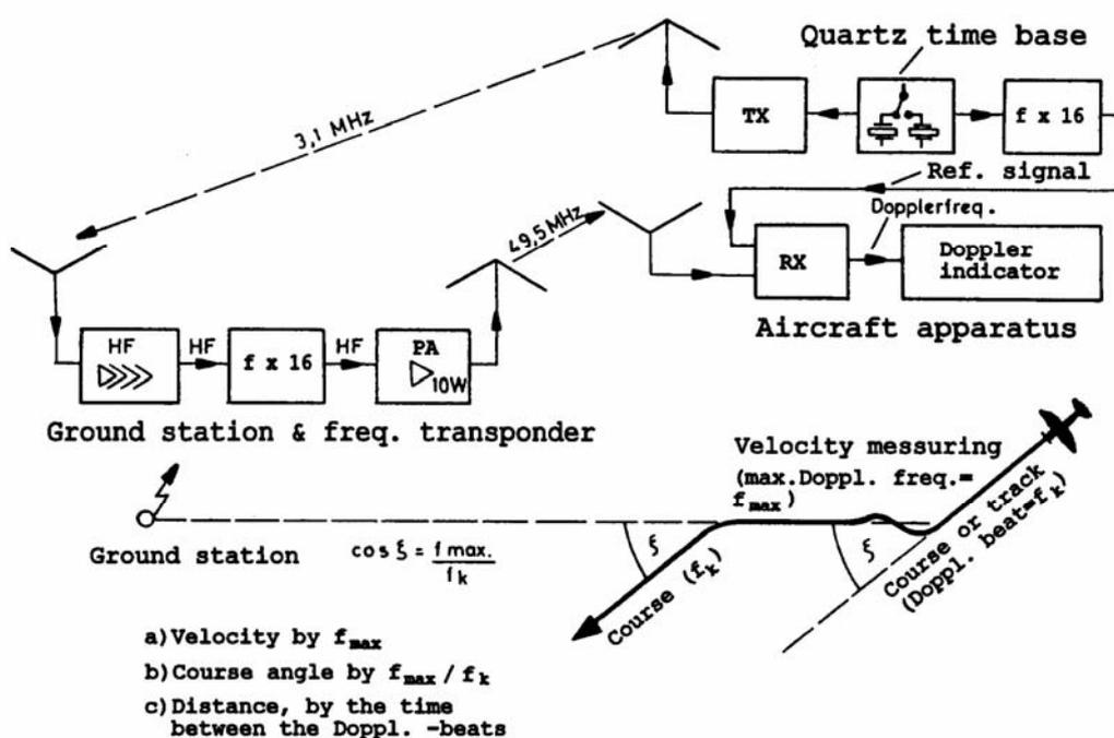
Figure 5: World's first operational aircraft Doppler-Navigation apparatus 1935/36 (DVL)
