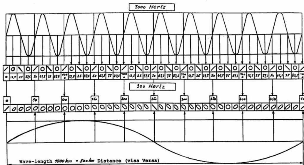
Figure 7: Signal phase – distance correlation as was used for Y- distance measuring
