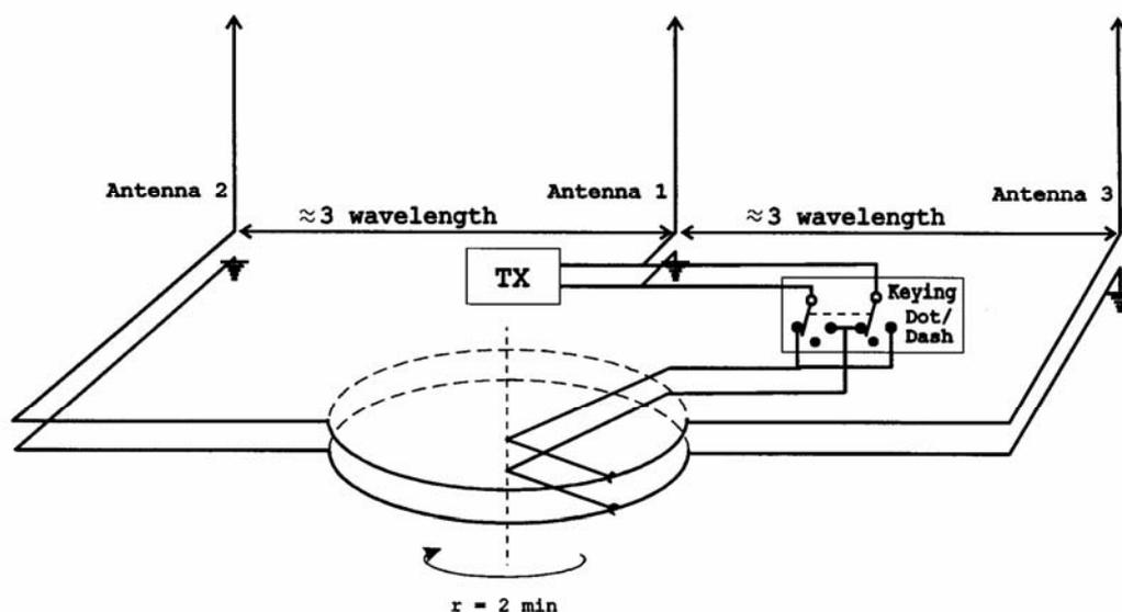
Figure 10: Simplified diagram of the Sonne or Consol apparatus
