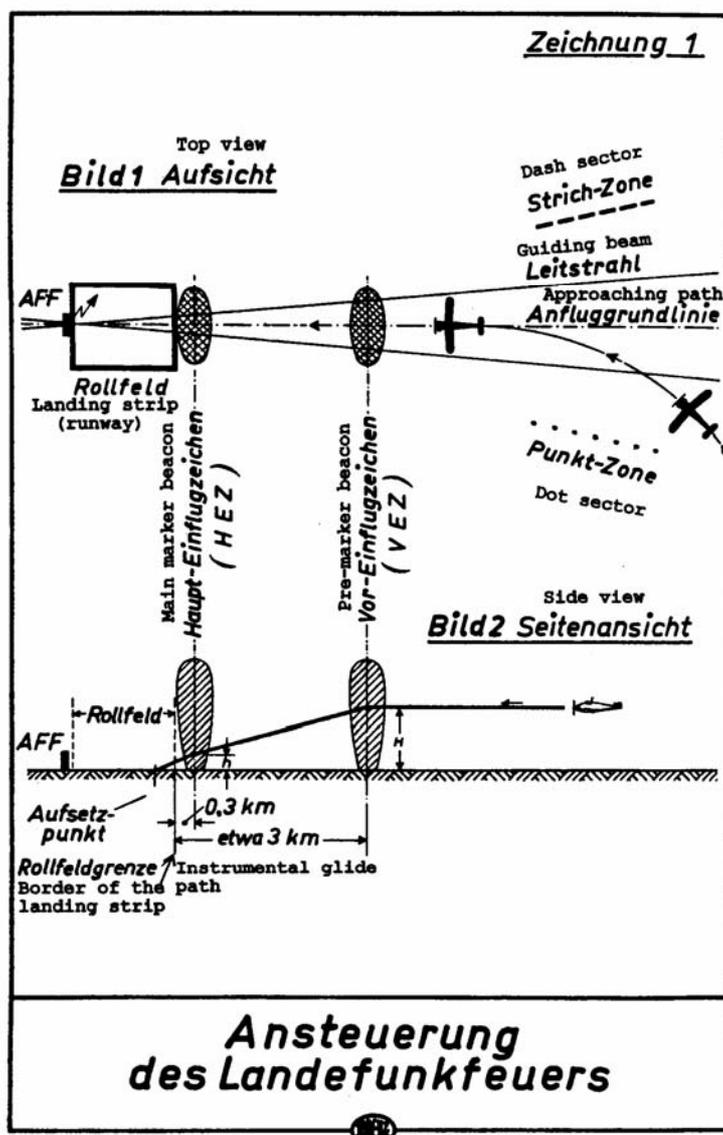
Figure 3: Lorenz instrumental B.A. system (Blindlandeanlage)
