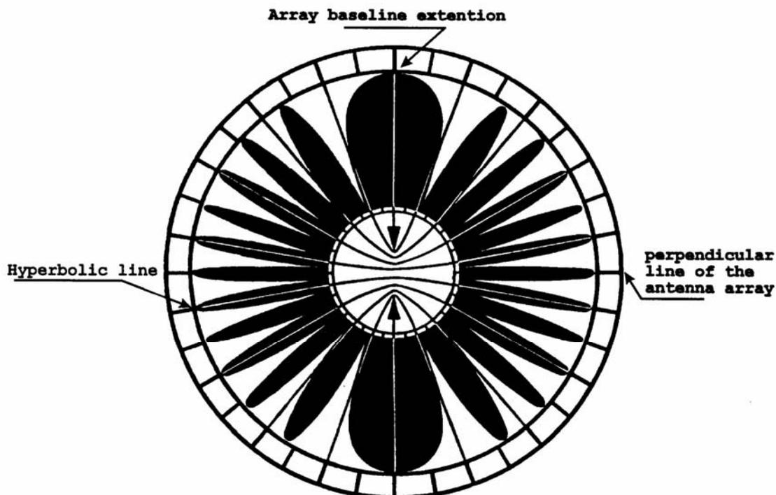
Figure 9: Radiation pattern of an antenna array of two vertical radiators, fed in phase, with a spacing of 6 wave-length, for the horizontal plain
