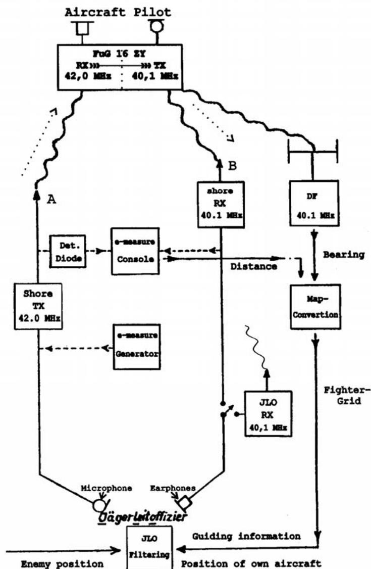
Figure 6: Operational e-measure guidance
