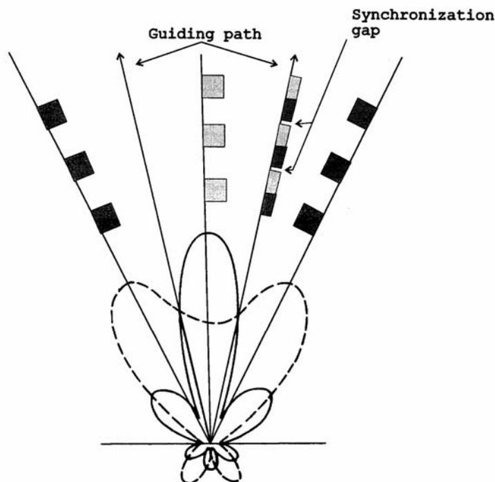
Figure 8: Dash – dash keying of the Y- beam
