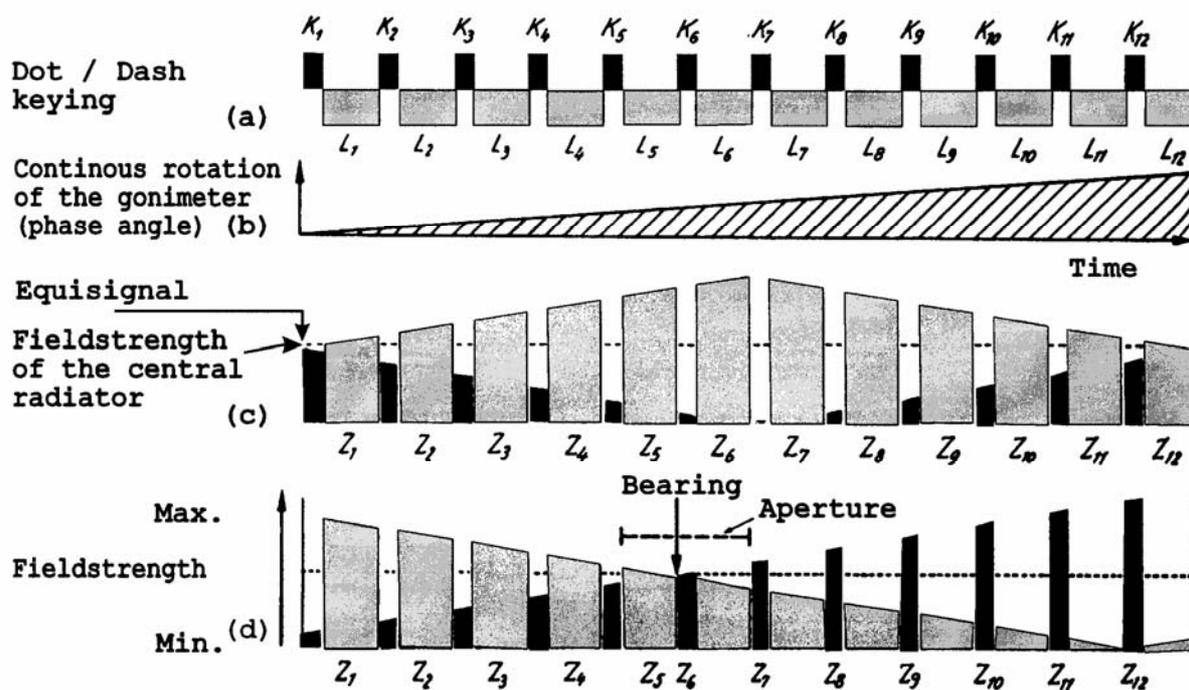
Fig. 11: Simplified dot/dash sequence of a Sonne or Consol system
