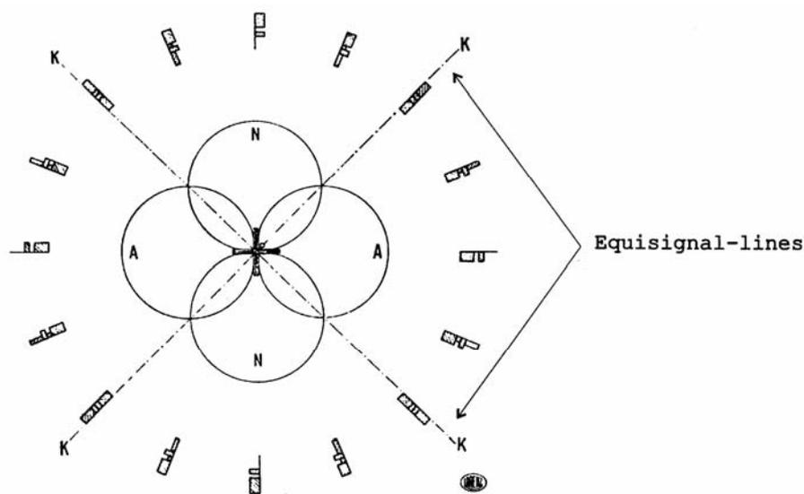
Figure 1: Scheller's virtual "A/N" path (1907) (Esau, [1, p. 348-349])
