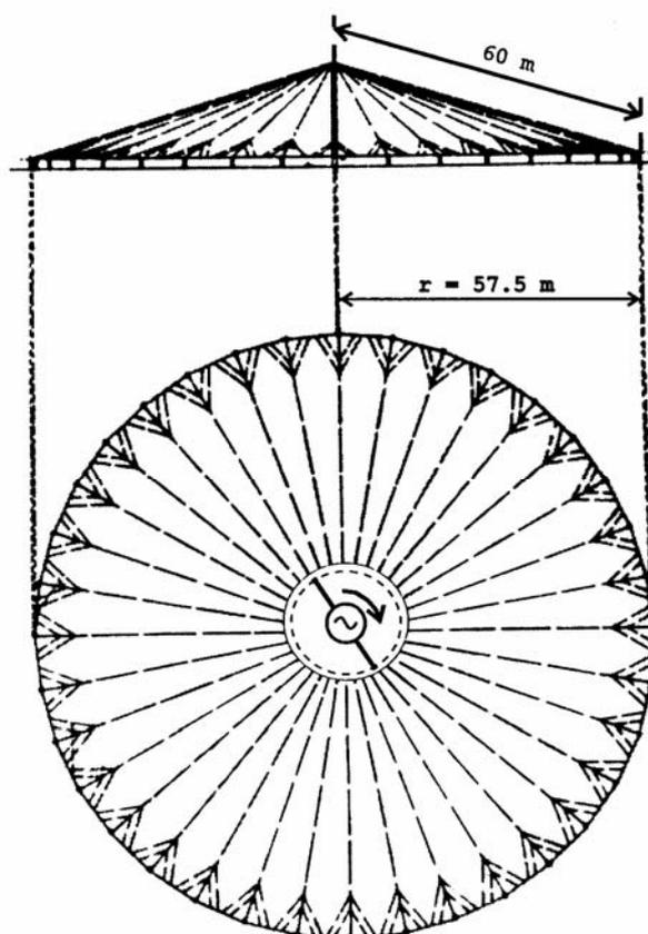
Figure 2: The antenna array of the Telefunken "Kompass-Sender"
