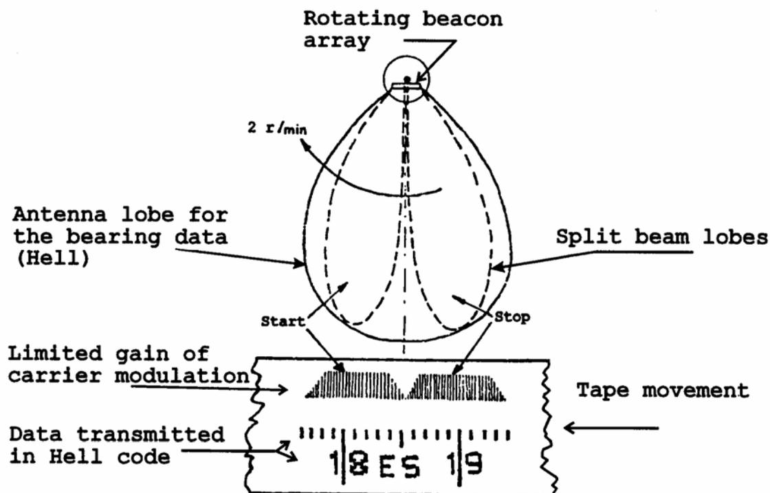
Figure 14: Bernhardine FuG 120a bearing, displayed on a paper tape, by a Hell printer device
