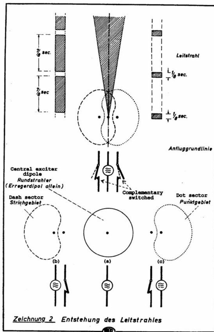
Figure 4: Beam forming of the virtual approaching path
