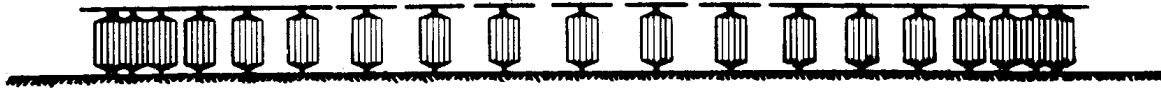
Figure 8: Wullenwever's horizontal view, we can see clearly why sine-law compensation is necessary
