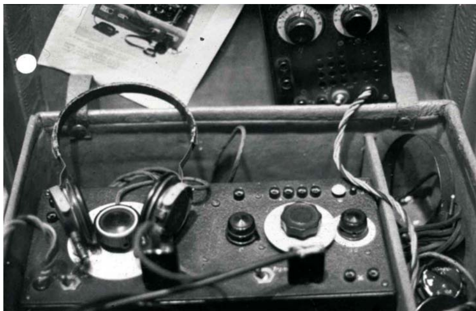
Figure 16 Until now, we have generally considered mains powered systems but, it is clear that battery powered stations were also operated. The type SE 92/3 (3 watt) was used in Western Europe as well as in Russia. For the latter theatre it was packed in a canvas cover. The
