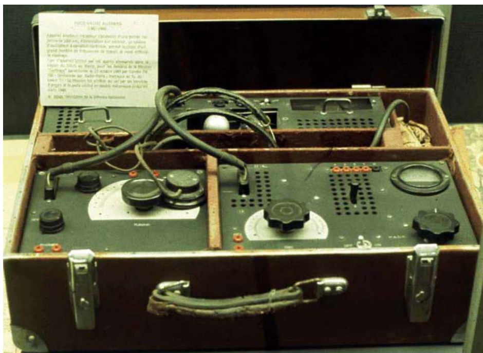
Figure 15 This portable suitcase station type SE 90/40 was fairly commonly in use by the Abwehr services on the European continent. The prefix SE means transmitter/receiver, drawing design-designation number 90, supplying 40 watts into the antenna. The left module contains the receiver and
